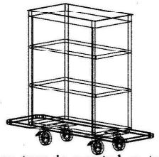
5. Upper tray is mounted on top of the side boards and back plate.
