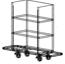
4. Back plate is fixed between the bottom plate and shelves with screws.
