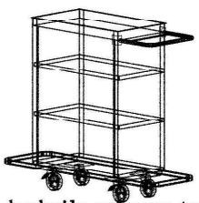
6, handrails and upper tray are fixed on the side boards with screws.
