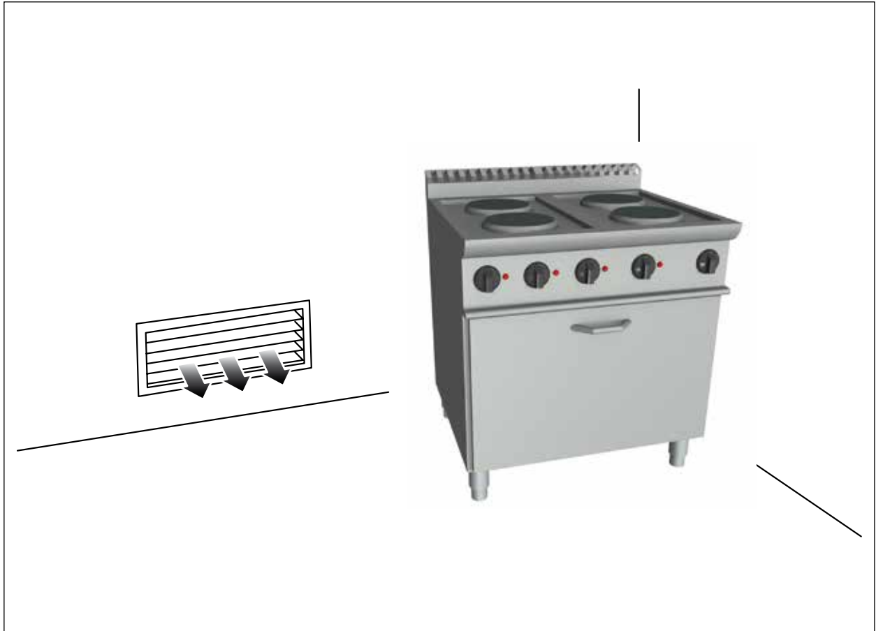
Fig. 21 Ventilation of the installation premises
